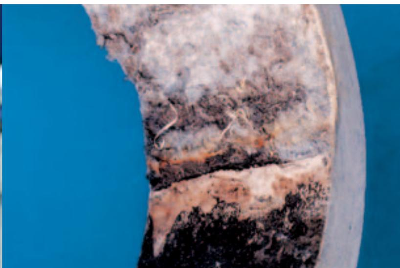
Costly: corrosion damage to a pressure pipe.
