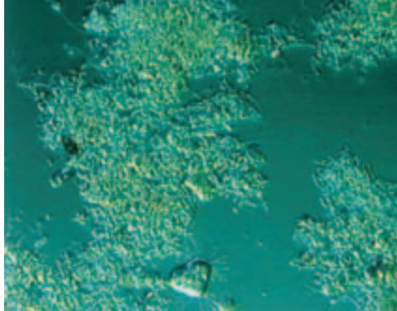
Well-developed sludge flocs after 14 days of oxygen treatment.
