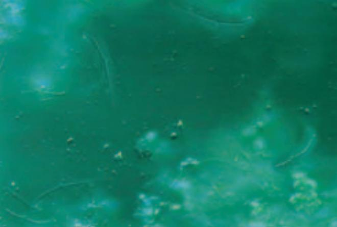
Weakly structured flocs caused by inadequate oxygen supply in the wastewater treatment plant of a brewery.
